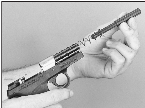
The disassembly tool is used to guide the slide over the recoil spring during reassembly. While the slide can be replaced without the tool, the process is easier with it in place.
