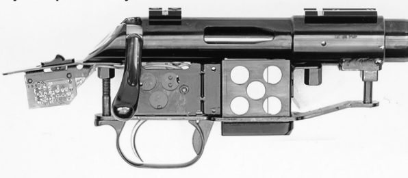
The VEC 95 RG's caseless ammunition requires an electronic ignition system powered by two 15V batteries.
